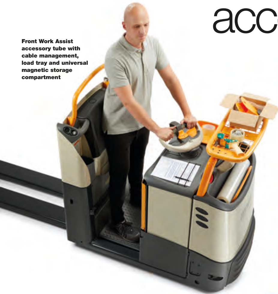
Front Work Assist accessory tube with cable management, large see-through clip pad and scan gun holder
