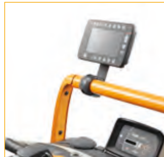
Front Work Assist accessory tube with cable management
